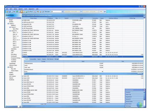
To see the details of a particular device, users simply click on the entry in the list to open a tabbed view with entries for counts, consumables, inputs, outputs and more.
